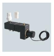
Uponor Fluvia T Push-12 mini pump groups for individual rooms and small heating surfaces. Room temperature regulation optionally via thermostat head with capillary room temperature sensor or Uponor room sensor (wire-based or wireless) with thermal drive. Ideal for connecting the radiant heating to an existing high temperature system.
