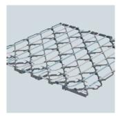
The Uponor Contec ON plastic special pipe carrier guarantees the exact height of the pipe in a level of a few millimeters above the ceiling underside. At the same time it acts as the spacer for the lower reinforcement.
