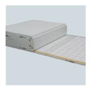
Uponor Klett roll panel – as the pipe fixation in rolled version with thermal and extra impact sound insulation to DIN EN 13163 and DIN 4108-10, made of EPS rigid foam with bondedon fabric adhesive foil for overlapping laying, with foil overlength selfadhesive on one side for covering the insulation layer in accordance with DIN 18560.
