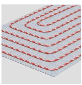
Uponor Klett Twinboard Ideal for fastening the Uponor Klett pipes to any existing floor insulation materials. The 2.4 m² large foldable hollow-chamber boards do not require much storage space, are easy to transport thanks to their low weight of only 1.9 kg and are very easy to work on the building site.
