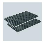
Uponor Tecto nub panel with insulation ND 11 or ND 30-2 with impact sound insulation. Pipe holding sheet plate made of EPS and backfoamed covering foil. For Uponor system pipes 14 – 17 mm. Laying spacing 10/15/20/25/30 cm.
