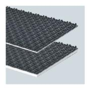
Uponor Nubos nub panel for rightangled and diagonal pipe laying in different pipe spacings. Optimal adaptation to existing room geometries with minimal waste cut through two-sided overlapping edge studs. Type ND 30-2 for universal usage in residential and commercial buildings up to 5 kN/m² Type ND 11 for service loads up to 30 kN/m².
