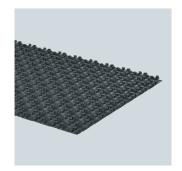
Uponor Nubos nub foil – for laying on existing insulation. Foil element without back-foaming. Vacuum-formed PS deep-drawn foil made of high-impact polystyrene with integrate pipe holder nubs for reliable observance of the pipe spacings and for exact height fixation of the Uponor system pipes.
