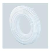
Uponor Minitec Comfort Pipe 9.9 mm with oxygen diffusion barrier made of EVOH. Colour natural with a blue stripe. Conforms to DIN EN: ISO 15875 "Plastic piping systems for hot- and cold-water systems, cross-linked polyethylene", oxygen tight to DIN 4726.
