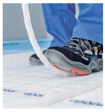
Uponor Klett is an innovative pipe fastening system for underfloor heating/cooling. The pipes have a Klett tape wound around them spirally. The suitable bonding foil is bonded across the entire surface on the system board. When the pipe is pressed onto the bonded board in the desired position, the Klett tape of the pipes then hooks into the adhesive foil of the insulation board with maximum holding force.
