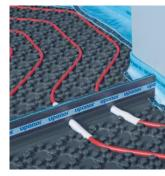
The Uponor Nubos wet construction system has been developed especially for underfloor heating/cooling systems in residential and non-residential buildings. The Uponor Nubos nub panels are installed in the floor structure below a load distribution layer made of cement or anhydrite screed and are available in three versions (ND 30-2, ND 11 and nub foil without insulation) for different floor structures and loads.
