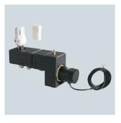
Uponor Fluvia T Push-12 mini pump groups for individual rooms and small heating surfaces. Room temperature regulation optionally via thermostat head with capillary room temperature sensor or Uponor room sensor (wire-based or wireless) with thermal drive. Ideal for connecting the panel heating to an existing high temperature system.
