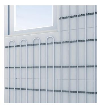
Uponor Fix is used in walls as a radiant heating/cooling system. The PE-Xa system pipes are integrated into the plaster, with the minimal plaster covering allowing very brief response times and thus rapid adaptation to changing operating states.
