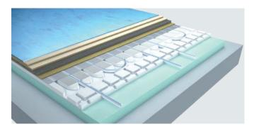
Uponor Siccus Sport floors are based on a 15-mm thick elastic layer made of permanently elastic special composite foam with high volume weight. The sports floors tested to DIN 18032 Part 2 attain their high stability through 2 offset load distribution panels
